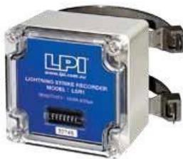
LPI® Lightning Strike Recorder (LSR1) is a lightning event counter. The LSR1 is simply mounted at any location along the downconductor route. It's purpose is to record the number of strikes captured by the lightning terminal and conveyed by the downconductor.
