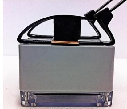
Figure 1: Mounting of LSR on HVSC down conductor    Figure 2: Mounting of LSR on flat down conductor
